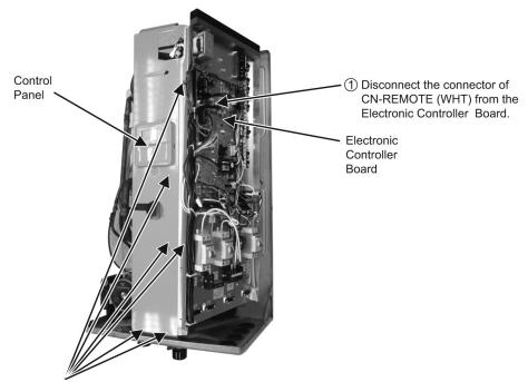
(2) Remove 6 screws to remove Control Panel.
