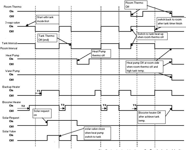
T1 = Backup heater delay time  $\pm$ ; 2 = Booster heater delay time
