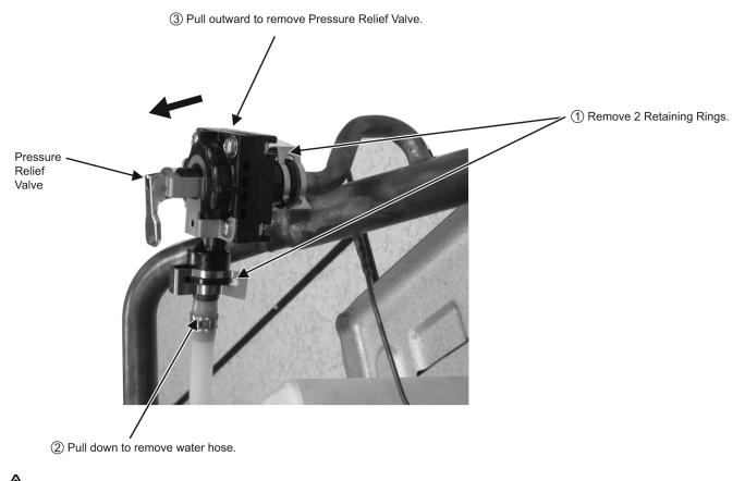
When reinstall the water pipe, use grease or water at the joining.
