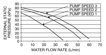
• Flow rate characteristic of indoor unit is as per above mentioned.
