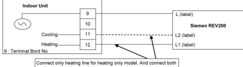
heating and cooling line for heat + cool model.
