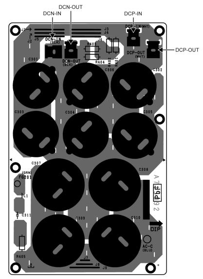
10.2.3. Noise Filter Printed Circuit Board
